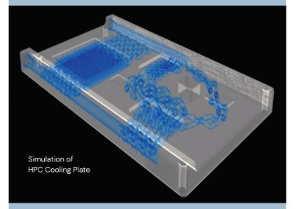
The suite of solutions includes multiple options for high performance designs engineered for low pressure drop, and optimal thermal performance.
