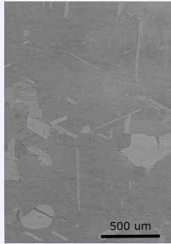
Figure 8: Microstructure of a bonded copper component's XZ plane showing five bonded feedstock sheets. No bond lines are visible in the microstructure.
